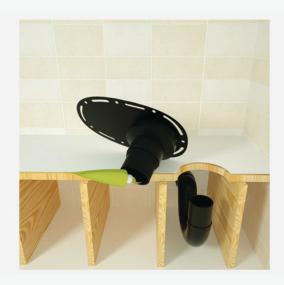
**3.** Connect the drain to the P-trap. Glue coupling reducer (if necessary) to the drain body first, then to the P-trap. Apply glue to both ends for a safe installation.
